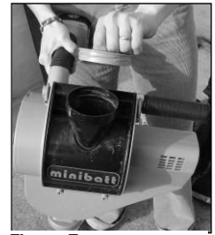
Figure 7 : Screw off full container
