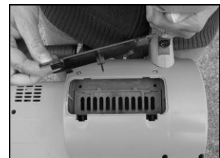
Figure 13 : Remove access disk
