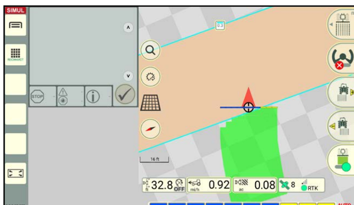
Fig. 250: Sections deactivated for headland and field boundaries
