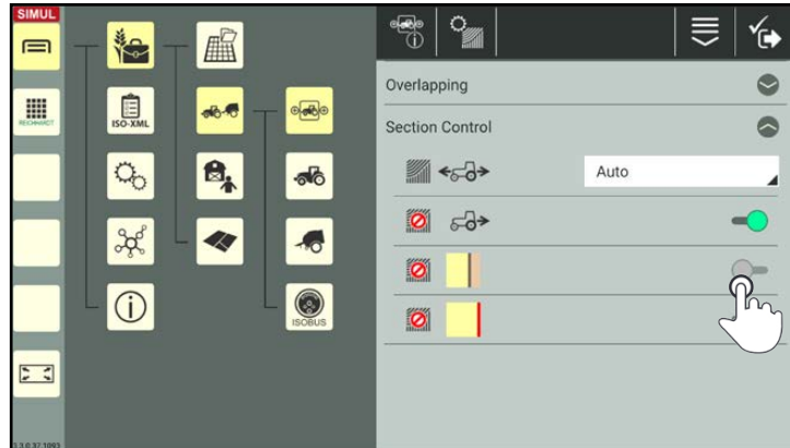
Fig. 253: Deactivating the switch to use section control in the headland boundaries
