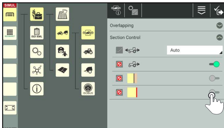
Fig. 255: Deactivating the switch to use section control beyond the field and headland boundaries
