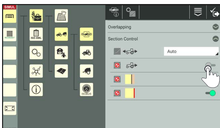
Fig. 252: Deactivating the switch to use section control when reversing
