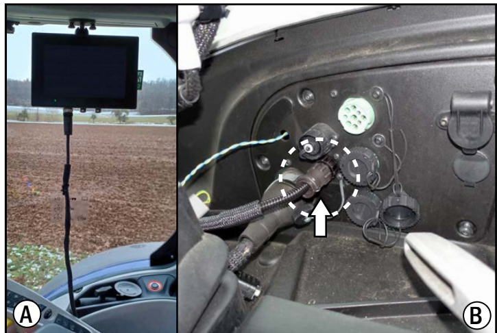
Fig. 12: Terminal connected to the vehicle's InCab socket
