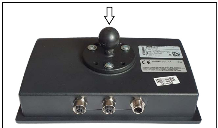
Fig. 9: Attach the RAM ball to the terminal
